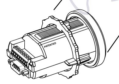
The gasket around the ring of the Link 10 should provide an adequate seal against moisture. If a sealant is used be sure it is **silicone** so that the Link 10 may be removed without damage.
